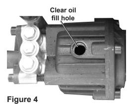
5. Look into the hole in the pump housing. If a metal wheel can be seen extending into the hole, SLOWLY pull the starter rope until the hole appears clear, as shown above.
